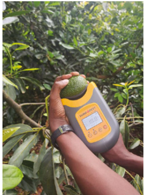
Portable, low-powered, battery-operated near-infrared (NIR) scanner.
