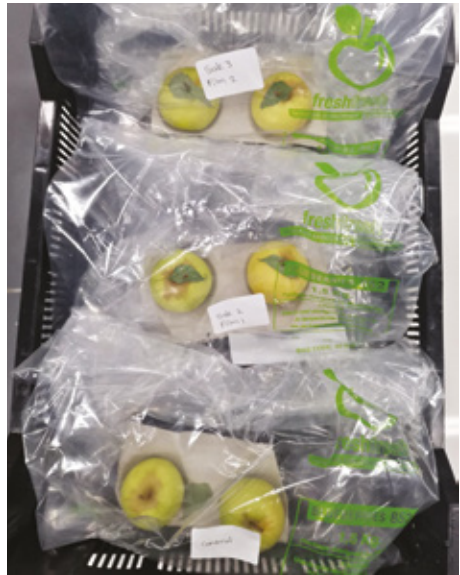
Modified Atmosphere Packaging (MAP) bags that help to determine the effects of modified atmosphere packaging on insect mortality and fruit quality
