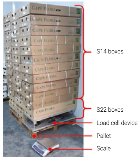
A device used to measure the loads on a palletised carton.
