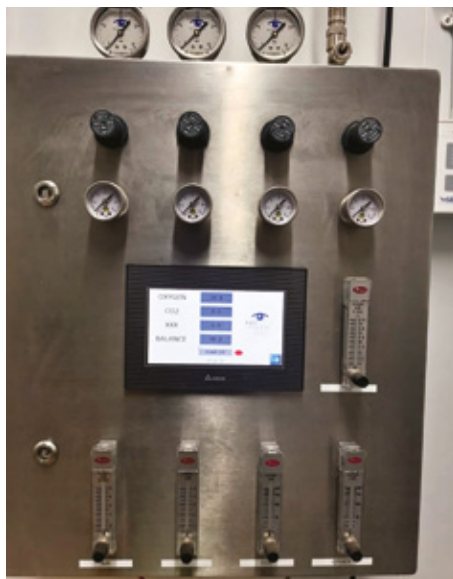
Mixing box to modify and measure gaseous composition in containers, e.g. oxygen, carbon dioxide and nitrogen levels. Fumigant and analyser can also be added to this system.
