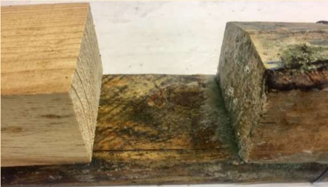
The pine block on the left has been treated with one of the products and shows no visual fungal contamination compared to the untreated pine block on the right.
