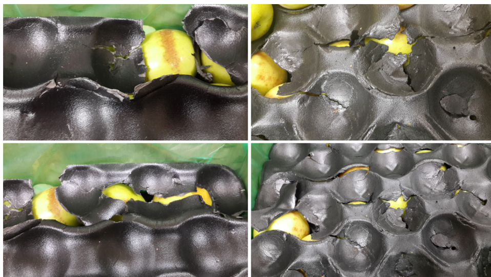
Fig. 11. Cracked trays after the vibration test.
